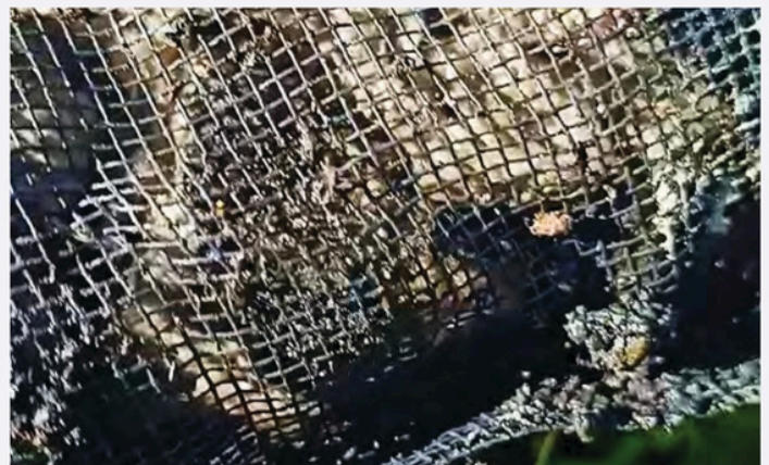
This sock shows dark areas where oils have been absorbed, as well as the light areas that show the basalt fibers can absorb much more.
