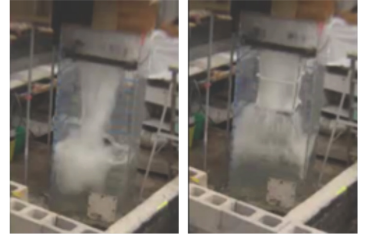
Standard catch basin and a catch basin enhanced with LittaTrap™.
