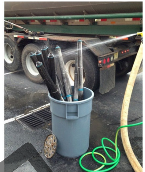
Rinsing of dirty filter cartridge tentacles with a low-pressure garden hose sprayer and using a plastic garbage container to capture rinse water.
