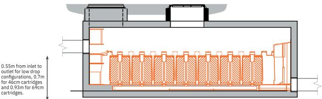
outlet for low drop for 46cm cartridges and 0.93m for 69cm cartridges.
