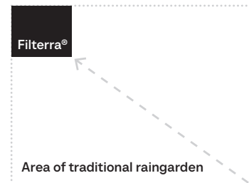
Based on a comparison of a traditional designed raingarden (k=0.3-0.75m/d) and the Filterra® (k=2.5m/d).
