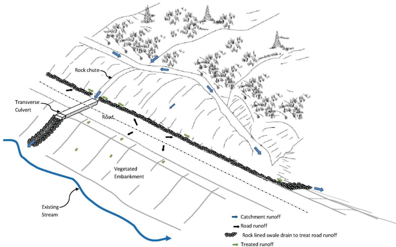
Figure 2 - Schematic of stormwater drainage elements within the road corridor
