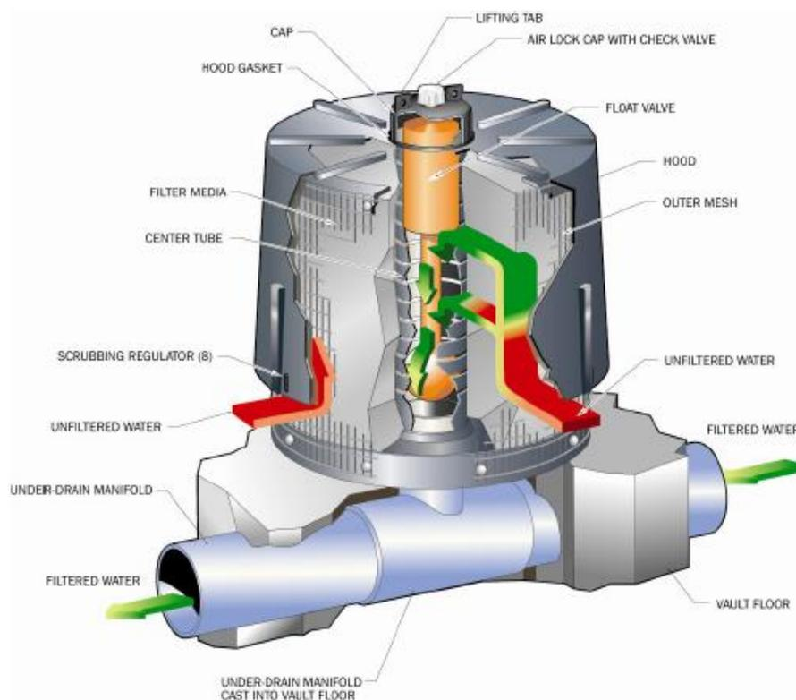
Figure 4: StormFilter Cartridge
