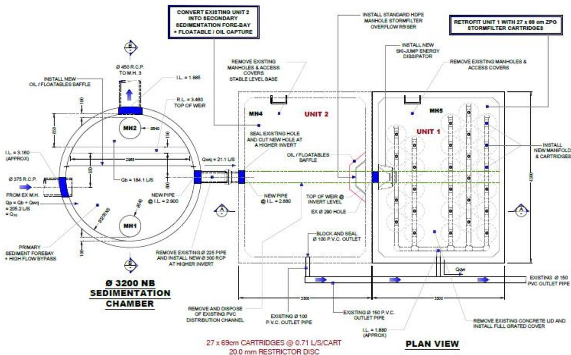
Figure 5: Retrofit (StormFilter) Layout Plan (Source: Stormwater360)
