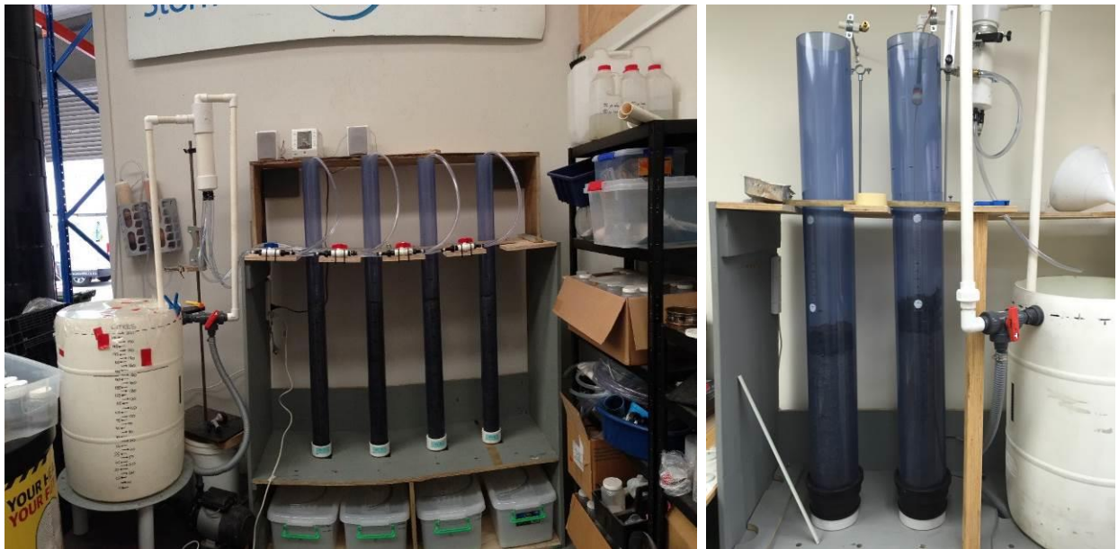
Figure 1 Four column laboratory test setup (left)
