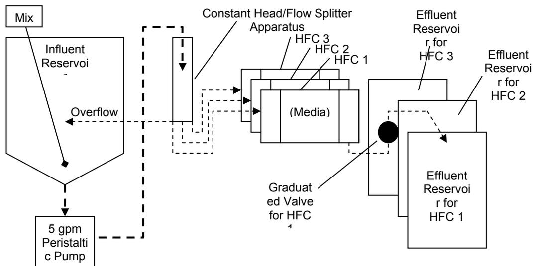
Figure 8: Schematic Laboratory Testing Apparatus
